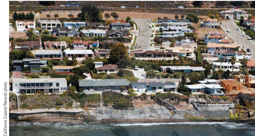
► FIGURE 13-51. These large homes sit atop a sea cliff without a beach in Pismo Beach in Southern California. Note that a new house is being built on the right, even though established houses have lost most of their yards and have spray cemented their cliffs to slow cliff loss.
