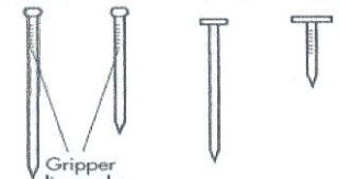
Gripper die marks Modern wire nails c.1850-present
